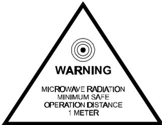
Figure 7 -1 The above label is attached to the TT-3007 Patch Antenna
