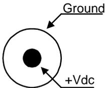
**Figure 7 -6: X1, Small DC Power input Connector**
