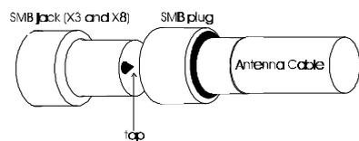
**Figure 7 -3: SMB jack and SMB plug**
