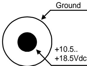
Figure 7 -7: X2, Large DC Power input Connector
