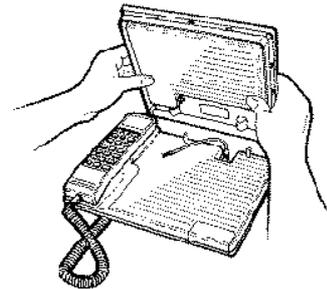
**STEP 3 Release the antenna stand from the frame.**
