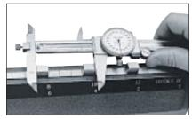
Checking accuracy of Dial Caliper using Caliper Checker.
