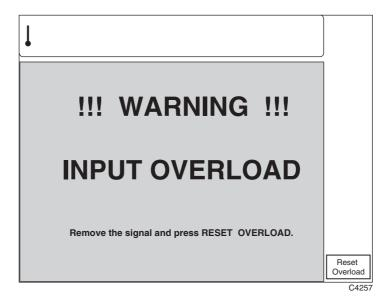
Fig. 3-8 Input overload warning screen
