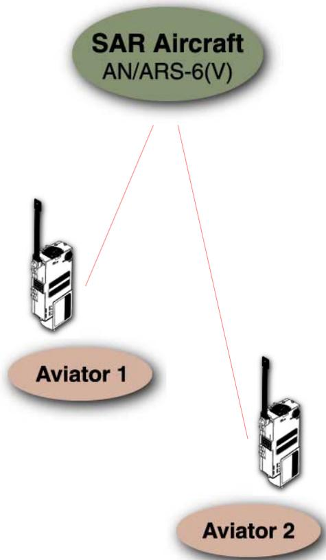
transmissions over Line-of-Sight paths. The Radio Set transmits amplitude modulated (AM) voice on 121.5 MHz, 243.0 MHz, 282.8 MHz, Channel A (predetermined programmed frequency), or Channel B (predetermined programmed frequency) as selected by the Radio Set Channel/Mode selector.
