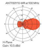
The Telewave ANT930Y10-WR Yagi is a high performance directional antenna, designed especially for point to point as well as point/ multipoint control applications. Seven elements provide a minimum of 10.5 dBd (12.6 dBi) forward gain, excellent front-to-back performance, and coverage of the entire 900 MHz commercial band. The boom and elements are solid 360° welded aluminum to prevent intermodulation and provide exceptional strength.
