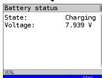
ARGUS indicates in the display when the battery is completely charged.
