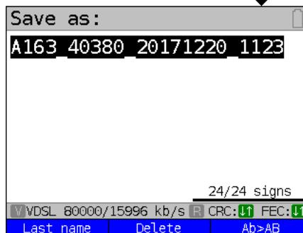
ARGUS saves the VDSL connection parameters together with the trace data in the first free slot. You can enter a user-definable name when saving (see page 290). ARGUS automatically suggests a save name, which is composed of:
