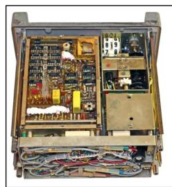
The UFT-435 was built extremely robust and rugged to withstand harsh field conditions. The operating temperature range of - 20°C to + 50°C and the degree of protection IP 54 (splash proof) secured the operability even in heavy rain and mud.
