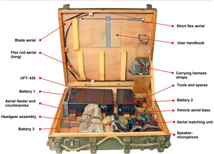
Layout of UFT-435 and associated components in transport case.
