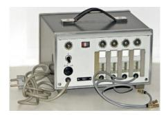
Battery charger LGT 7, type number 85 248, for charging four UFT-435 batteries.
