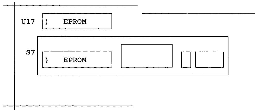
When replacing these devices, ensure that the replacements marked CB-S7 and CB-U17 are fitted to the correct sockets and that the pin orientation is correct as identified by the semi-circles in the above drawing.
