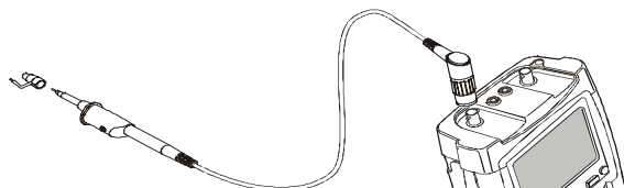
Figure 37. HF Voltage Probe Connection Using Ground Spring
