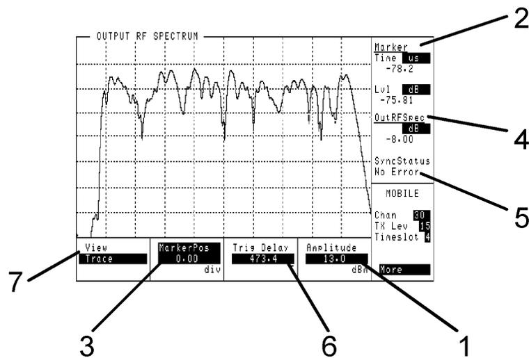
This view displays output RF spectrum power spectral density (at the Freq Offset setting) versus time.
