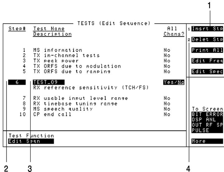
Figure 8-15 Edit Sequence Screen on the HP/Agilent 83212X
