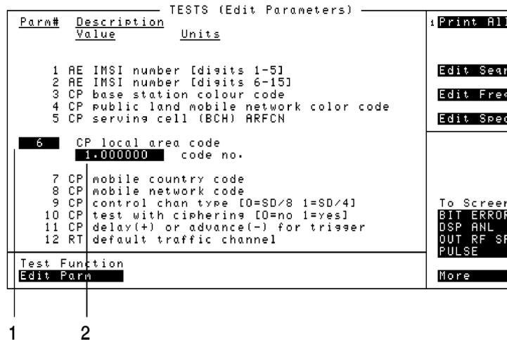
**Figure 8-16 Edit Parameters Screen on the HP/Agilent 83212X**
