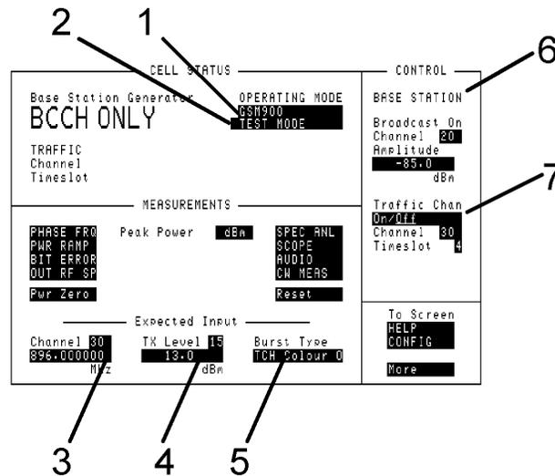
This screens allows you to test the mobile phone without a call being set up.
