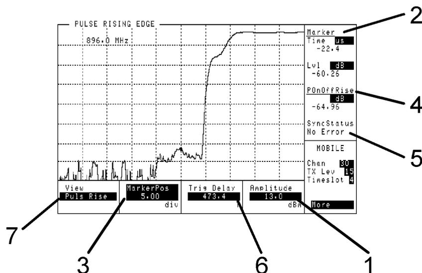
This view displays Pulse On/Off power spectral density versus time for the rising portion of the burst.
