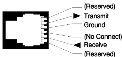
**13. SYSTEM BUS** The system bus connector is used to externally control frequency hopping and contains duplications of several individual connectors.
