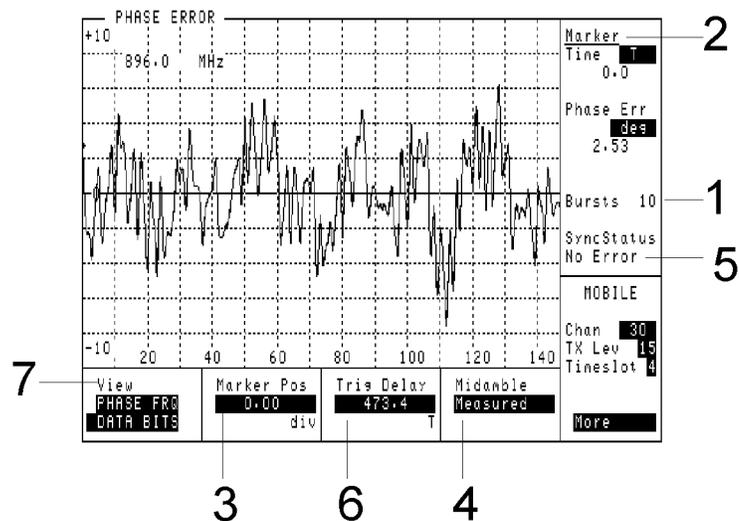
This view displays phase error versus time. The vertical range is scaled to the measurement. The horizontal range is 0 to 147 or 0 to 87 bit periods depending on the burst type.
