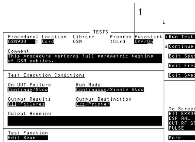
Figure 8-13 Tests Screen of the Agilent 8922M/S
