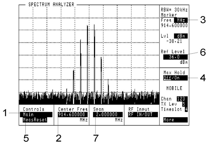
This screen displays the Spectrum Analyzer power spectral density versus frequency trace.
