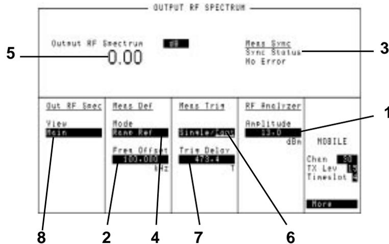
The Agilent 8922M/S uses a 3-pole synchronously tuned filter to make Output RF Spectrum measurements rather than a 5-pole filter as specified in the GSM recommendations. Refer to Section titled “Output RF Spectrum Measurements Using a 3-Pole Synchronously Tuned Measurement Filter” in Chapter 2.
