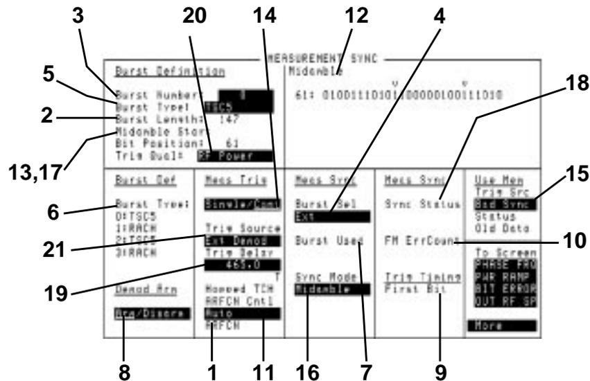
This screen defines settings that determine how synchronization will occur for any of the following measurements:
