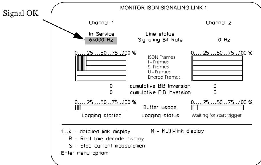
**Agilent 8922M** To log protocol messages into the Agilent 8922M
