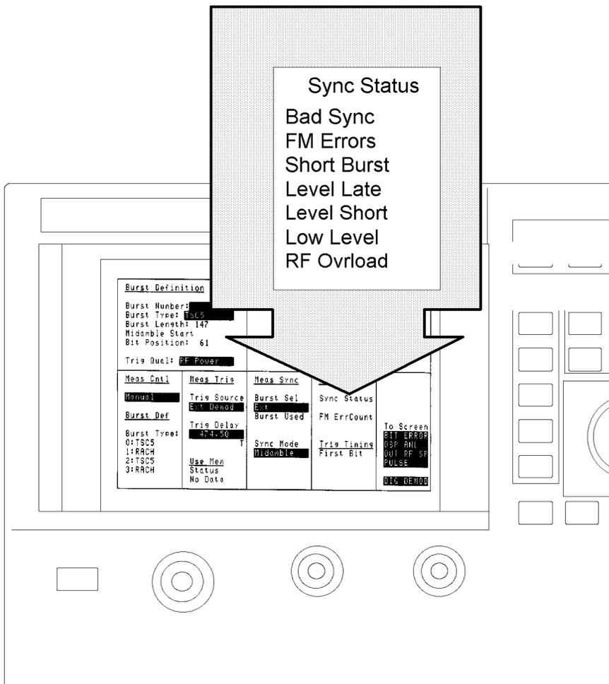
**Possible Solutions to Sync Status Errors**    **Solution 1 - Trigger Timing**
