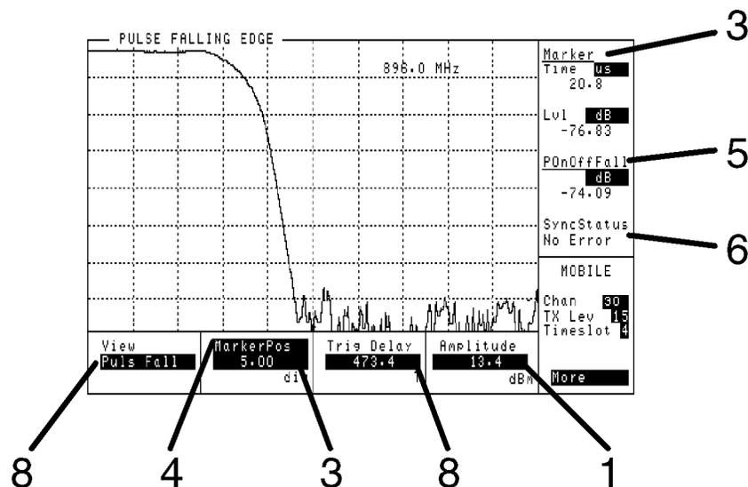
This view displays Pulse On/Off power spectral density versus time for the falling portion of the burst.
