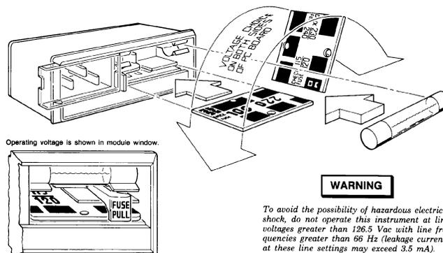
1. Open cover door, pull the FUSE PULL lever and rotate to left. Remove the fuse.
