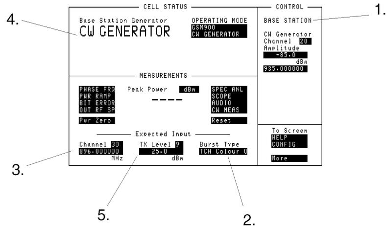
This screens allows you to set the Agilent 8922M/S up as a CW Signal Generator.
