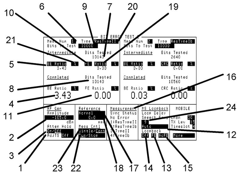
Each time the Bit Error Test is run, four measurements are made (see Meas Num). Because of limited screen space, only two measurements are displayed at one time. The upper left side of the screen will display measurement 1 or 3, and the upper right side will display measurement 2 or 4. For further information, read the field description for Meas Num.
