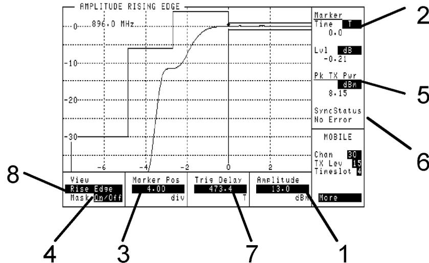
This view displays the rising portion of the amplitude envelope with the amplitude mask superimposed. The vertical range is -40 to +5 dB. The horizontal range is -8 to +4 bit periods.
