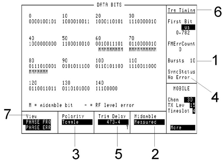
This screen displays the measured demodulated data bits and tags indicating how each bit was interpreted by the measurement.
