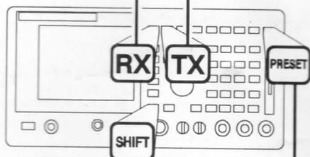
Use this key to activate the blue labeled functions. Press and release, then press the key below the blue label.
