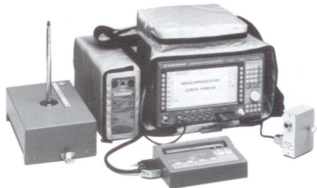
CMS33 inclusive options: External battery, VSWR head, remote control box and the front cover with antenna
