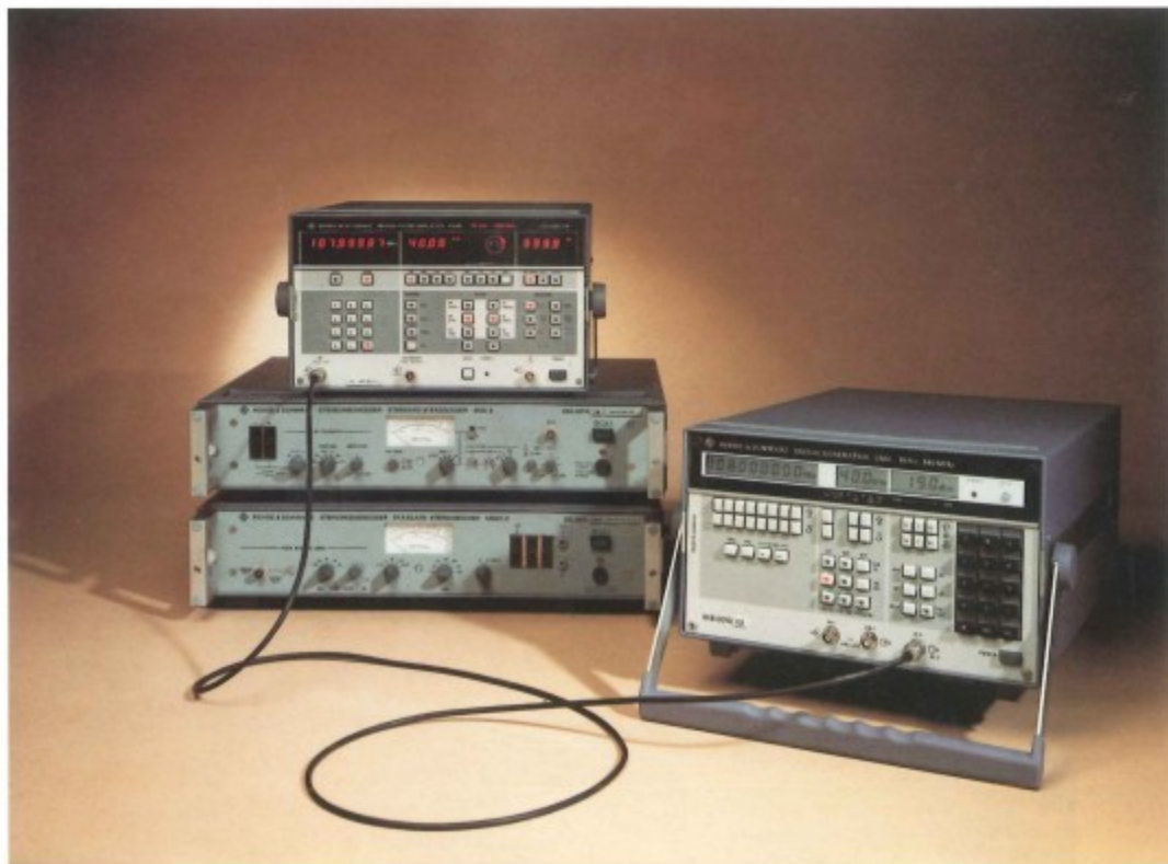
With Signal Generator SMK, Modulation Analyzer FAM, Precision Stereocoder MSC 2 and Stereodecoder MSCD 2, R&S offers a complete set of equipment for stereo measurements
