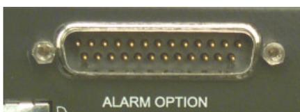
Figure 2.7: Alarm Relay Card Rear Panel
