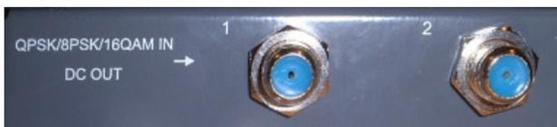
Figure 5.3: QPSK Input Card Rear Panel
