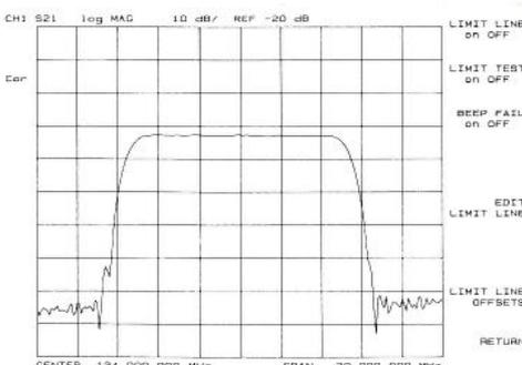
In this example, we enter a [**STIMULUS VALUE**] of 127 MHz (at the start of the filter passband), an [**UPPER LIMIT**] of -21 dB and a [**LOWER LIMIT**] of -23 dB. The SAW filter under test has about 22 dB insertion loss in the passband. Terminate this segment by selecting [**DONE**]. Since this is a flat limit segment select [**LIMIT TYPE**] and [**FLAT LINE**] (the default type). Select [**PRIOR MENU**] to return to the limit line edit menu.
