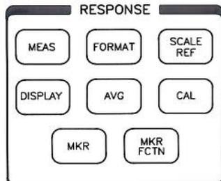
The network analyzer's receiver section is controlled with these keys. The top three keys allow the user to choose measurement configuration (A, B, B/R, etc.), presentation format (amplitude and phase versus frequency, Smithchart, polar coordinates, etc.), and scale and reference values for a full screen display.
