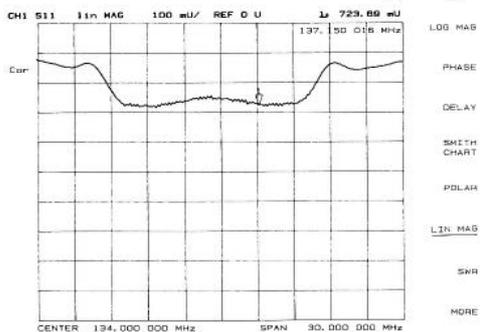
To display the same data in terms of reflection coefficient, press **[FORMAT][LIN MAG]**. This simply redisplay the existing measurement in a linear magnitude format that varies from  $\Gamma = 1.00$  at the top of the display (100% reflection) to 0.00 at the bottom of the display (perfect match).
