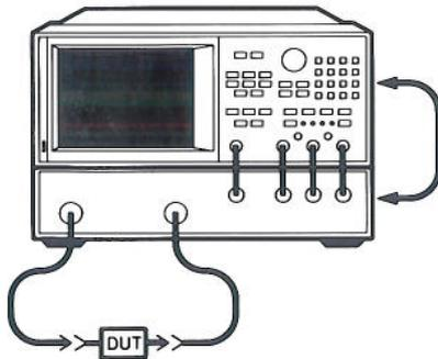
Connect the S-parameter test set to the network analyzer as explained in chapter 1, "Installation"
