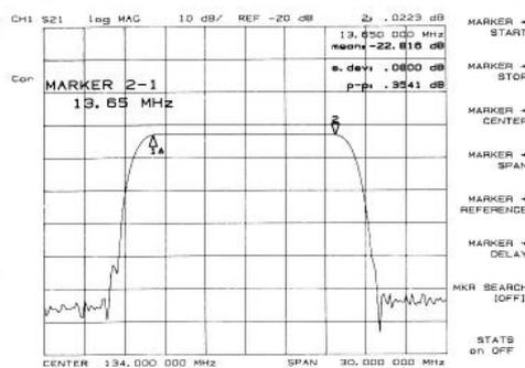
The power of marker statistics is illustrated in this measurement of passband ripple. Passband ripple (or flatness) is the variation in insertion loss over a specified portion of the passband.
