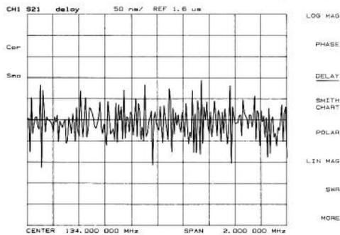
The default aperture is the frequency span divided by the number of points across the display (i.e. 201 points or 0.5% of the total span in this example). Other aperture values can be selected by turning on [SMOOTHING] and varying the [SMOOTHING APERTURE] in the [AVG] menu.
