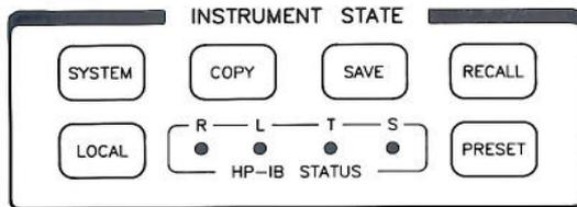
Several utility functions are implemented with these keys, including instrument preset, front panel save/recall memory, HP-GL plotter control, time domain transform (optional) and built-in diagnostic tests.
