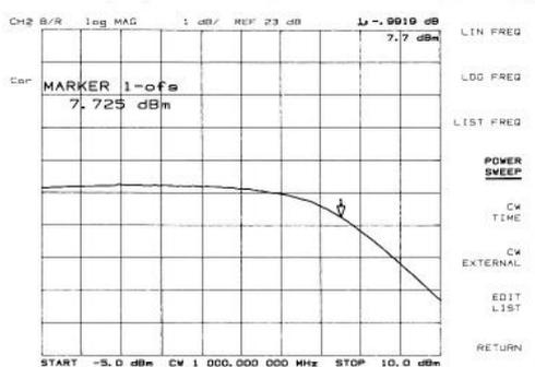
The figure shows the gain rolling off as the input power increases to a level where the amplifier under test exhibits gain compression. While the +20 dBm maximum output from the network analyzer will be sufficient for many compression tests, it is also possible to add an external amplifier in series with the source to provide additional drive. Remember to limit the input power to the analyzer to 0 dBm maximum, adding external attenuators if necessary.
