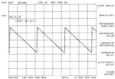
The above setup results in the phase response measurement shown. Note that the SAW filter under test has considerable phase shift within only a 2 MHz span. Other filters may require a larger frequency span to see the effects of phase shift.
