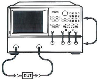
A two input ratio measurement can also provide information about the phase shift or insertion phase of a network. The HP 8753C can translate this information into a related parameter, group delay.
