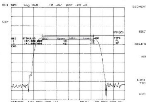
You are now ready to do limit testing. Select [**DONE**] to return to the limit menu. The analyzer draws the limit lines on the display when you select [**LIMIT LINE ON**]. Select [**LIMIT TEST ON**] to activate the limit test. The analyzer tells you whether the DUT passes or fails the limit test with a message along the right hand edge of the graticule. Select [**LIMIT TEST OFF**] and [**LIMIT LINE OFF**] when you are finished with this measurement.
