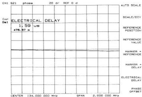
1. Activate the line stretch function by pressing **[SCALE REF]** **[ELECTRICAL DELAY]**.
