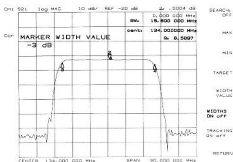
The HP 8753C calculates the bandwidth of the DUT between two equal power levels. In this example, we calculate the  $-3$  dB bandwidth relative to the filter center frequency.
