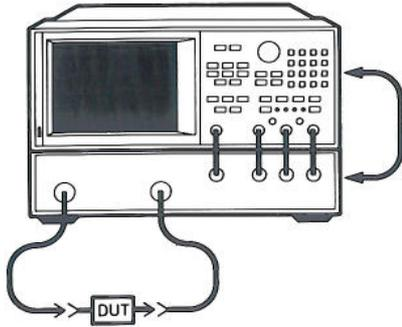
Connect the S-parameter test set to the analyzer as shown. The DUT will be the SAW filter used previously.
