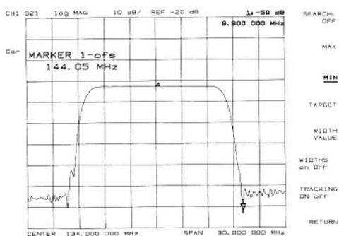
The wide dynamic range of the HP 8753C allows it to measure stopband rejection up to 110 dB below the pass band response. As discussed in chapter 6, "Increase Dynamic Range", maximum dynamic range requires proper selection of input power level, IF bandwidth and averaging.
