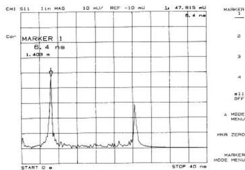
Press [MKR] and use the knob to position the marker on the reflection of interest. Note that the marker reads the time and distance to the reflection in the upper left hand side of the graticule. Loosen one of the connectors to see the corresponding reflection increase.
