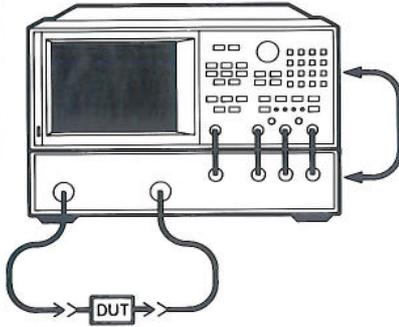
Group delay is the transmission time through the DUT as a function of frequency. Mathematically, it is the derivative of the phase response which can be approximated by the ratio
