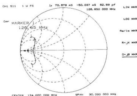
Use the marker to read admittance parameters. From the **[MKR]** menu, select **[MARKER MODE MENU]** and **[SMITH MKR MENU]**. Note that the default selection (currently underlined) is **[R + jX MKR]** for impedance marker readout. Select **[G + B MKR]** for an inverse Smith chart overlay. The marker reads the admittance data in the form  $G \pm jB$ , where  $G$  is conductance and  $B$  is susceptance, both measured in units of Siemens (equivalent to mhos).
