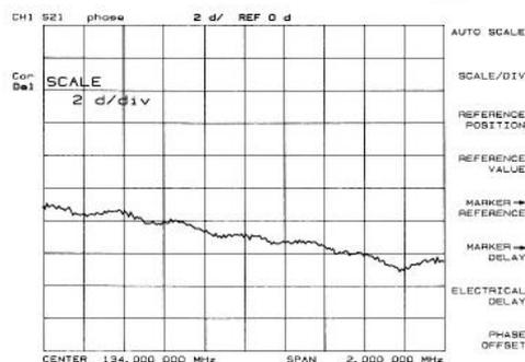
This can be measured using the previous setup for measuring electrical length. By adding electrical length to "flatten out" the phase response we have removed the linear phase shift through the DUT. What remains is the deviation from linear phase shift through the device. Simply increase the scale resolution to directly measure the deviation from linear phase.
