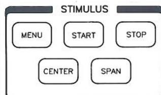
These keys allow the user to define an appropriate source output signal for the device under test. Source frequency may be swept over any portion of the range 300 kHz to 3 GHz, at power levels between +20 and -5 dBm. The Stimulus keys can also control the start and stop times in the (optional) time domain mode. The choices for sweep time and resolution, linear versus logarithmic sweep, power sweep, etc. are also selected here.
