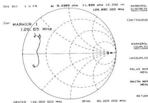
The display shows the complex impedance of the DUT over the frequency range selected. Press **[MKR]** and use the knob to read the resistive and reactive components of the complex impedance at any point along the trace. Note that the marker annotation tells that the complex impedance is capacitive in the bottom half of the Smith chart display and is inductive in the top half of the display.
