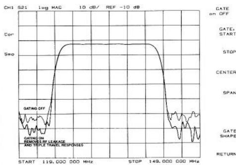
Time domain analysis also lets you mathematically remove individual parts of the time domain response to see the effect of potential design changes. We do this by "gating" out the undesirable responses. In the example shown to the left we see the effect of removing the RF leakage and the triple travel signal path using gating. By transforming back to the frequency domain we see that this design change would yield better out-of-band rejection for the SAW filter under test.
