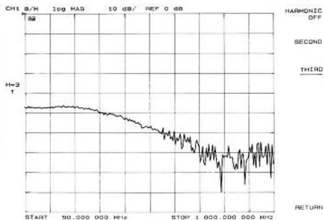
Third harmonic mode [*THIRD*] displays the preamplifier's third harmonic response relative to the fundamental (dBc).
