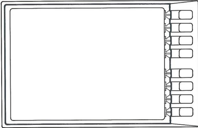
One of the more noticeable characteristics of the HP 8753C is the simplicity of its front panel. Rather than individual keys for each of the many instrument functions, the analyzer uses CRT-displayed "menus" for operator input. These menus list the possible choices for a particular function, with each choice corresponding to one of the eight "softkeys" located to the right of the CRT.
