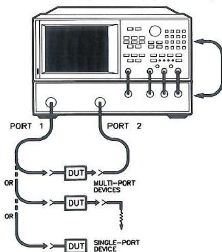
Connect high quality terminations (loads) to all unused ports. With an S-parameter test set, measurement port 2 supplies this termination during measurements of  $S_{11}$  and  $S_{21}$ , while port 1 supplies the load for measurements of  $S_{12}$  and  $S_{22}$ . All switching is automatic, controlled by the analyzer. When using a transmission/reflection test set, terminate the unused port at the B input of the analyzer or with a high quality load.
