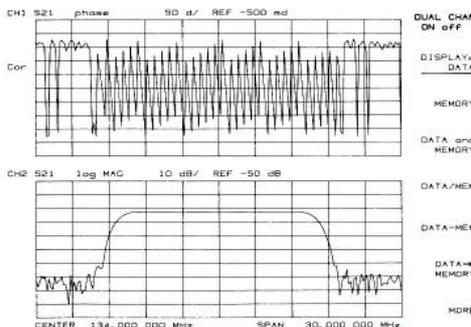
In some cases it is useful to be able to view more than one measured parameter at a time. Simultaneous gain and phase measurements for example, are useful in evaluating stability in negative feedback amplifiers. Such measurements are easily made using the dual channel display.
