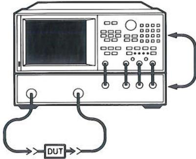
The HP 8753C electronically implements a function similar to the mechanical "line stretchers" of earlier analyzers. This feature simulates a variable length lossless transmission line, which can be added to or removed from a receiver's input to compensate for interconnecting cables, etc. In this example, the electronic line stretcher is used to measure the electrical length of a test device.
