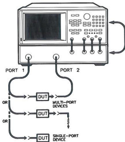
These parameters are really no different from the measurements made in the previous section.  $S_{11}$  is the complex reflection coefficient of the DUT input, while  $S_{22}$  is the complex reflection coefficient of the DUT output. In both cases, all unused ports must be properly terminated.
