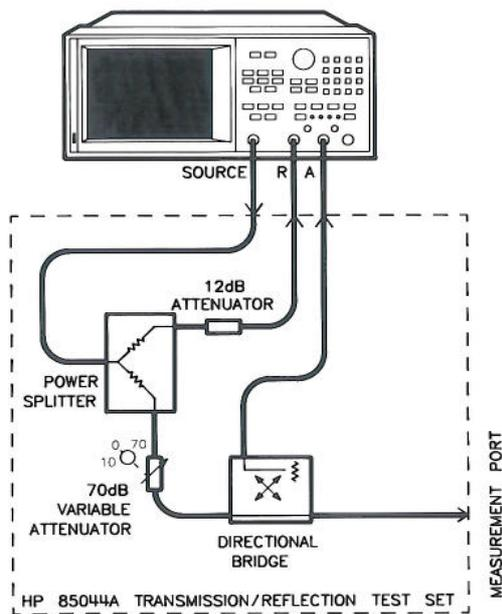
As shown in the diagram, the HP 85044A/B test set contains the hardware required to make simultaneous transmission and reflection measurements in the forward direction. The only setup required is to connect the DUT input to the test port and the DUT output to the B input of the analyzer. The HP 85044A is a 50 ohm test set and the HP 85044B is a 75 ohm test set.
